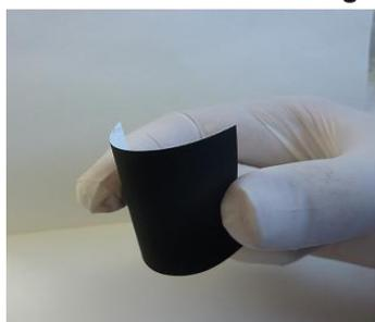
Figure 2a : Image of printed cathode electrode
